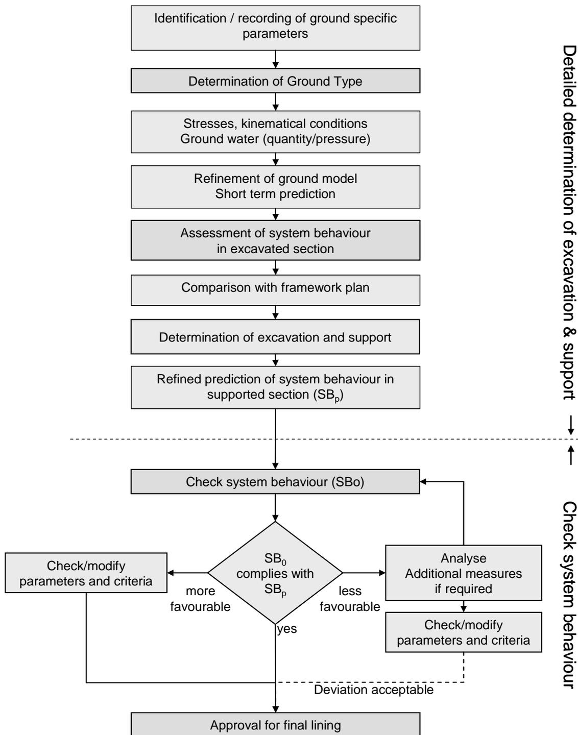
Figure 3: Basic procedure of determination of construction measures and check of system behaviour during construction ( $SB_p$  = predicted system behaviour,  $SB_o$  = observed system behaviour)
